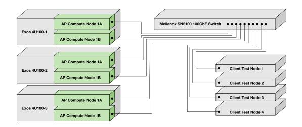
The network topology leveraged one of the two 100GbE ports offered by the Mellanox dual-port HBAs. While we tested configurations that placed server peer-to-peer communications on ports physically separate from the test client paths, we did not see an appreciable change in throughput. A bonded network configuration was not tested.
