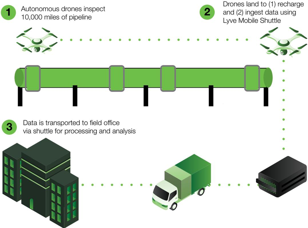
Thanks to advancements in asset-maintenance technologies today, midstream companies can conduct remote inspections using autonomous drones that capture high-resolution images of pipelines. Engineers can run analytics on these photographs to identify rust, corrosion, or other pipeline-integrity indicators.
