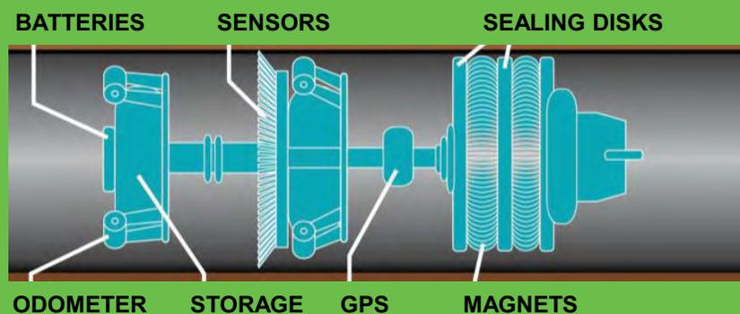
Capturing and transferring the tremendous datasets PIGs generate is a feat. Typically, a PIG will travel 100 miles over the course of two days before a worker removes it, using a special trap to capture data. After that distance, PIGs typically generate up to 400GB of unstructured data. Over the course of a 10,000-mile trip, a PIG can produce as much as 41TB of data; over 2,000TB (or 2.1PB), each year.
