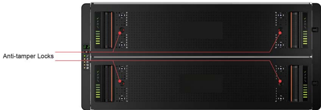
Figure 6-1 Anti-tamper Locks (shown disengaged)
