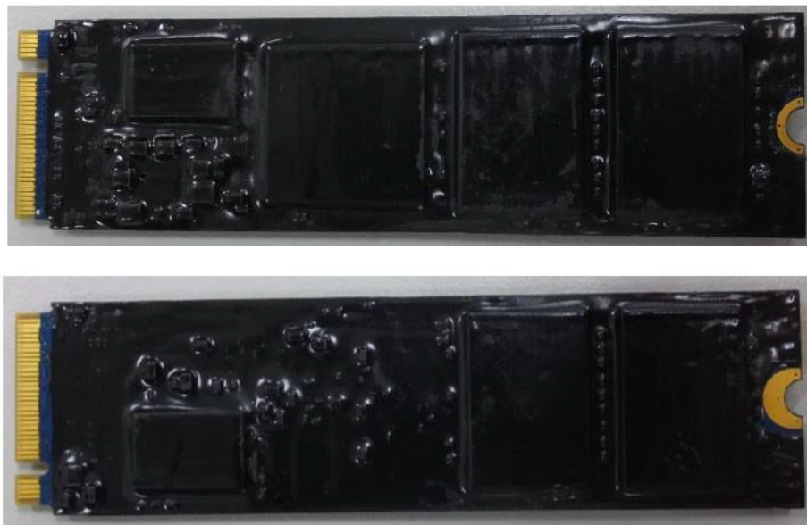
Figure 5 Example of FIPS tamper-evident epoxy resin
