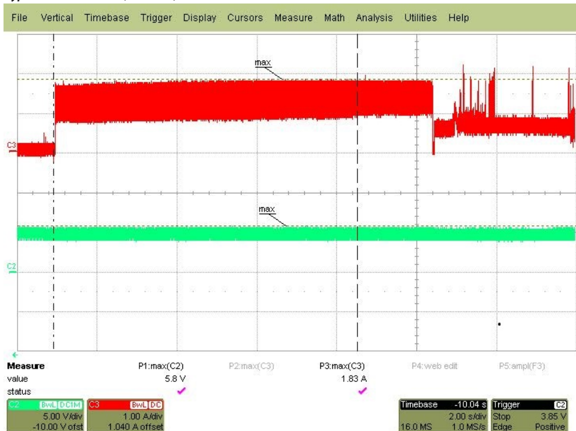
Figure 1 Typical Current Profile (5V & 12V)
