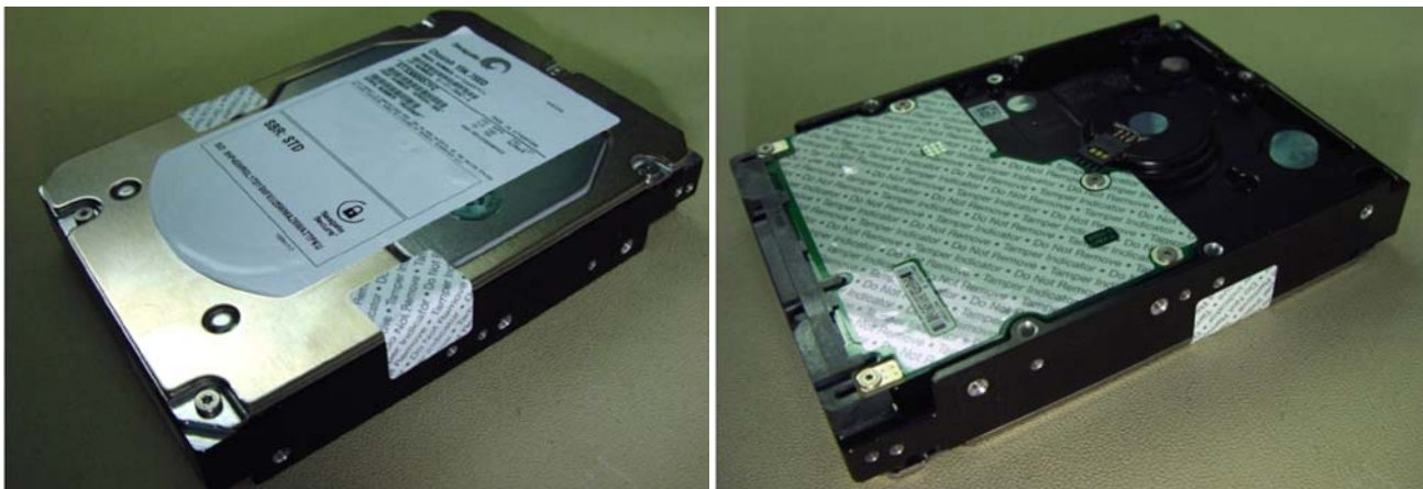
Figure 10. Example of FIPS tamper evidence labels.
